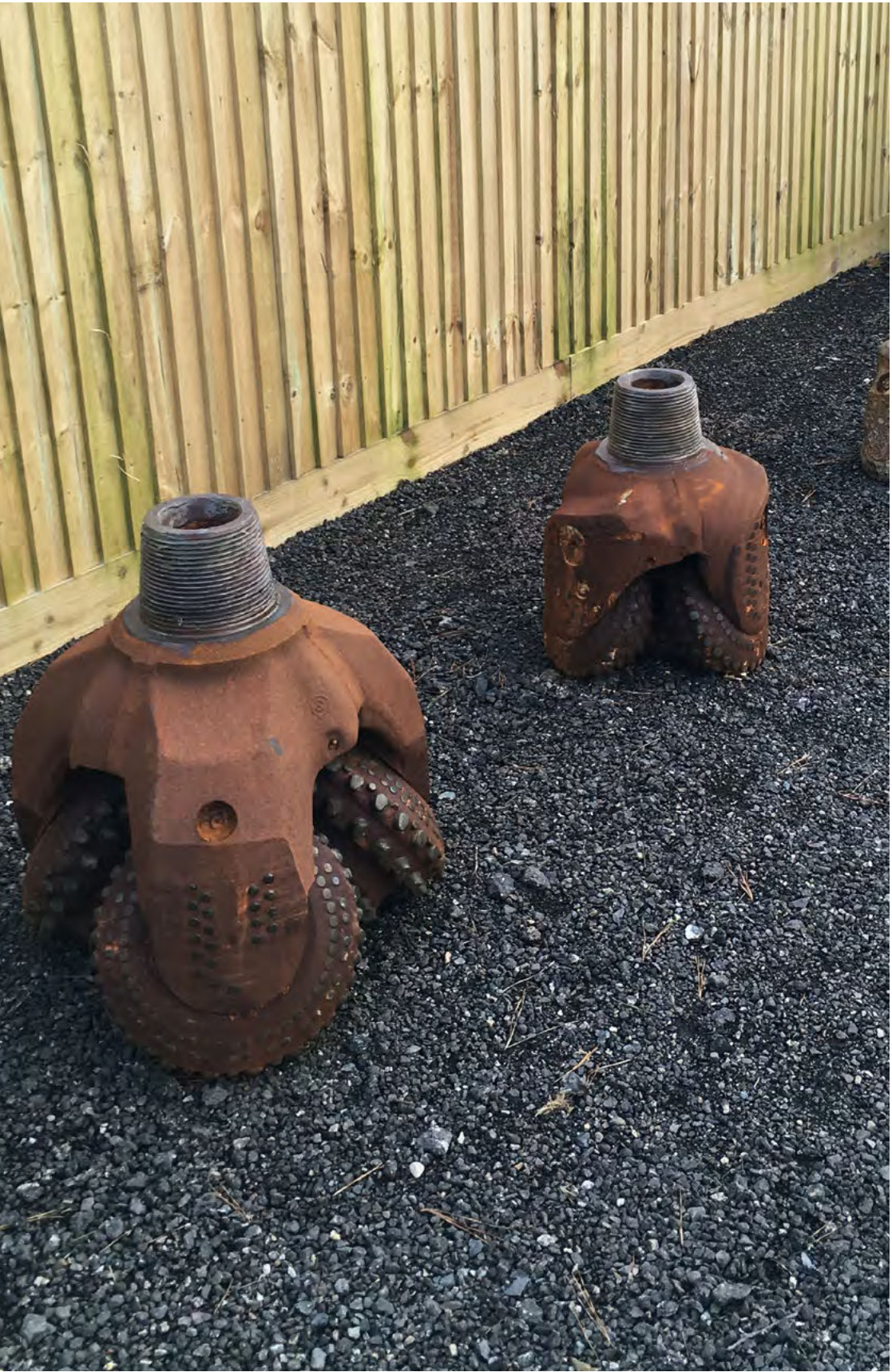
Steel tri-cone drill bits with tungsten carbide inserts used for drilling the United Downs boreholes Courtesy of GEL
